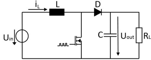
Fig. 7. Boost converter circuit.
