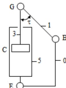
Fig. 7. The transmission angle ( $\tau$ ) in the elevation subsystem.
