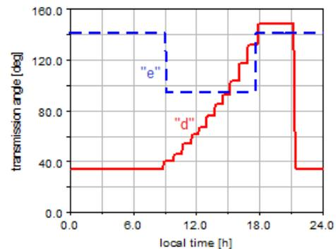
Fig. 11. The transmission angles in the tracking mechanism.
