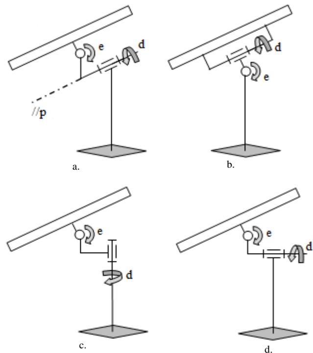
Fig. 1. Dual-axis tracking mechanisms.
