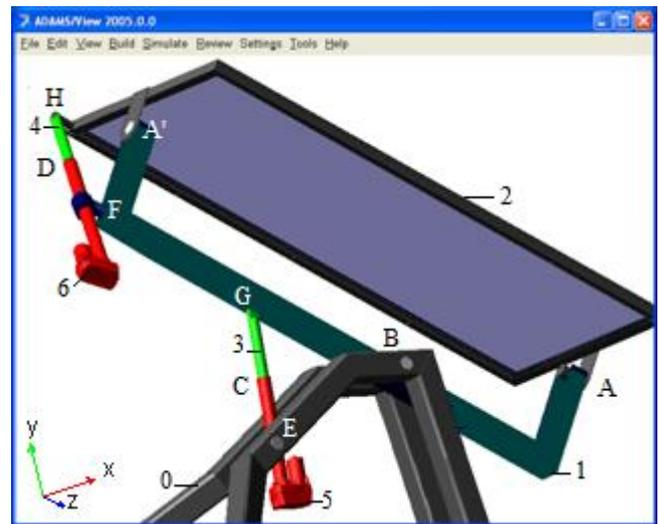
Fig. 2. The MBS model of the mechanical subsystem (ADAMS).
