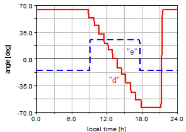
Fig. 8. The dual-axis tracking program.
