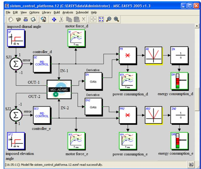
Fig. 6. The DFC model of the control subsystem (EASY5).
