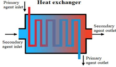
Fig. 2. The operating principle of heat exchangers.
