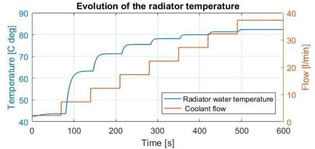
Fig. 5. The nonlinear behavior of the coolant temperature in the radiator at different flow values.
