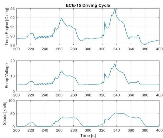
Fig. 8. Rejection of disturbances by the control system using ECE-15 driving cycle.
