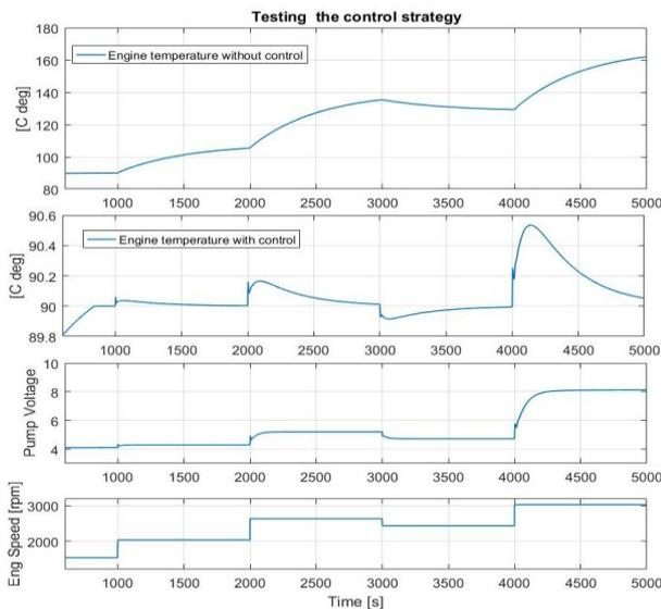
Fig. 7. Rejection of disturbances by the control system for different engine speeds.
