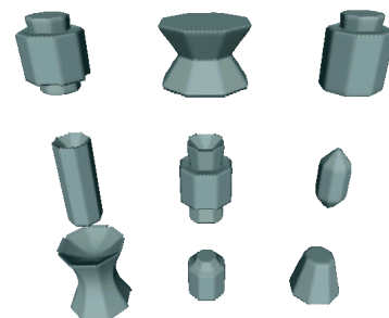
Fig. 6. Implicit spherical product surfaces m(x, z) \otimes h(x, y) = 1 defined by using the curves in Fig. 5(A)-(I) as m(x, z) = 1 and the curve in Fig. 5(K) as h(x, y) = 1 .
