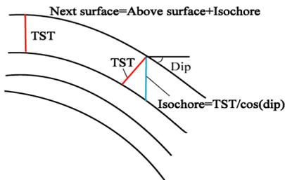
Fig. 5. Schematic chart of isochore and reservoir planes calculation
