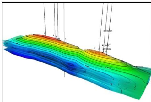
Fig. 8. Structural model with the boreholes positions
