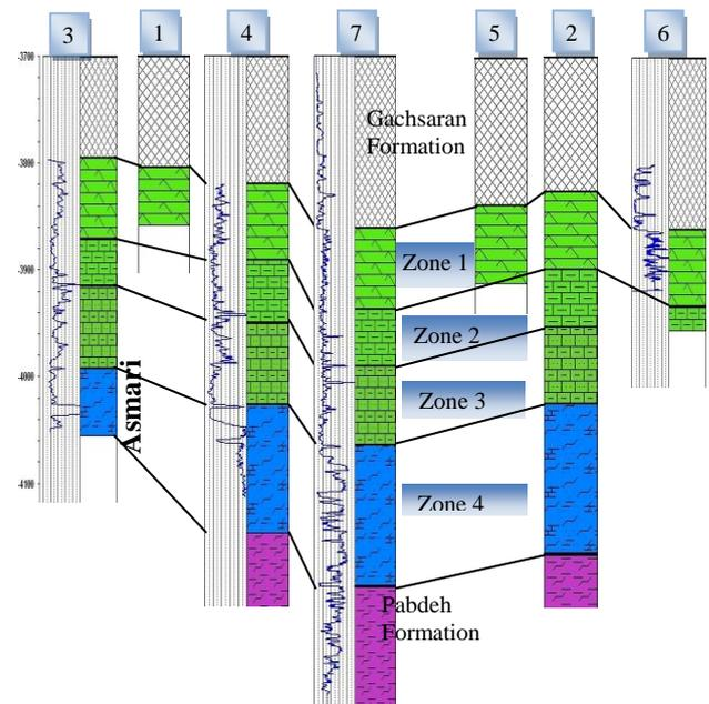
Fig. 2. Stratigraphic correlation chart of the Asmari reservoir zonation in drilled wells.
