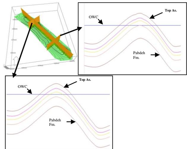
Fig. 9. Different structural latitudinal sections representing a smooth anticline.
