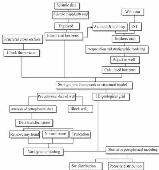
Fig. 1. Schematic flow chart of the petroleum reservoir modeling steps
