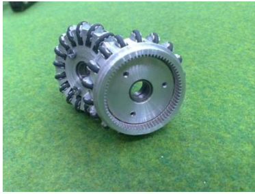
Fig. 2. Real omnidirectional wheel
