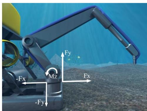
Fig. 7. Interaction forces between the ROV and the manipulator.
