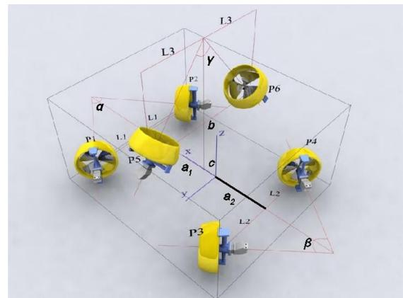
Fig. 6. ROV Thrusters position scheme
