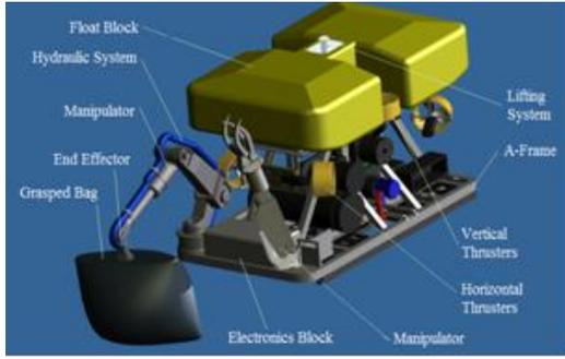
Fig. 1. ROV "Quark" with a manipulation system
