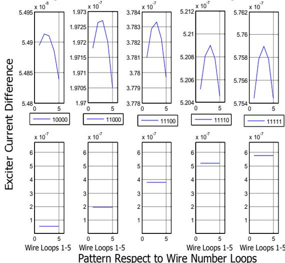
Fig. 7. Pattern changes with fixed defect value for 5-loops case with increased defect at each loop with movement exciter scan with 75Hz
