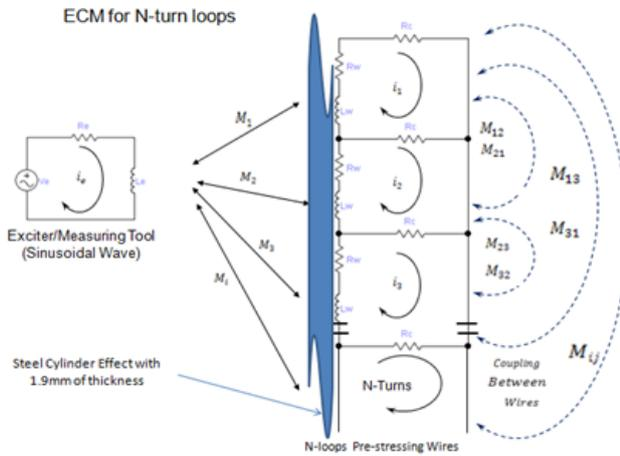
Fig. 4. Equivalent circuit model for PCCP
