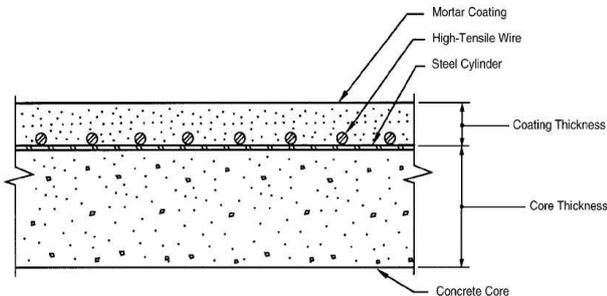
Fig. 2. The cross section and elements of Embedded Cylinder Pipe (ECP) [3]
