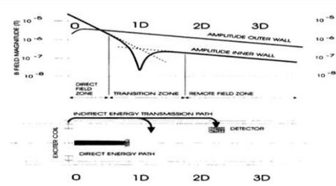
Fig. 8. Shows the B field magnitude profile inside and outside the pipe
