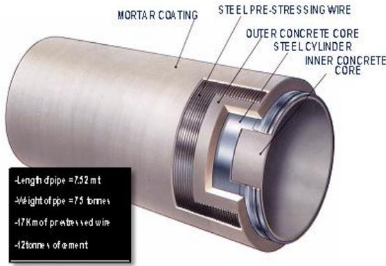
Fig. 3. PCCP material components
