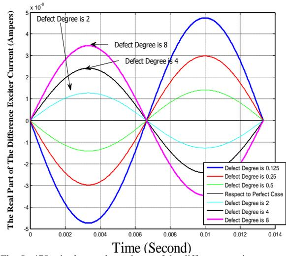
Fig. 5. 478-wire loops: the real part of the difference exciter current with different defect values degrees with exciter at loop 1 with frequency of 75Hz.
