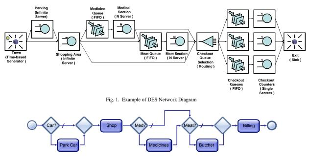
Fig. 2. Example of BPMN diagram
