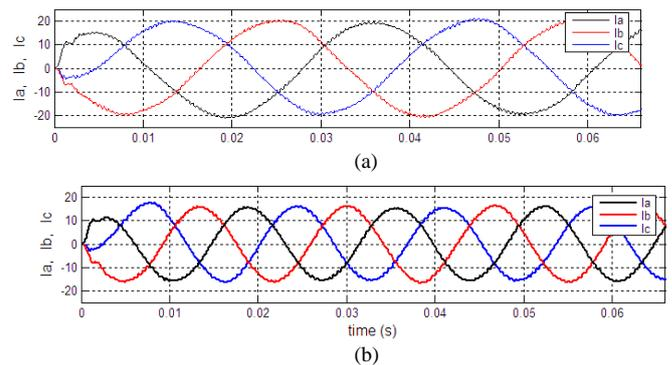
Fig. 8. Three phase output current: (a) in 30 Hz (b) in 60 Hz
