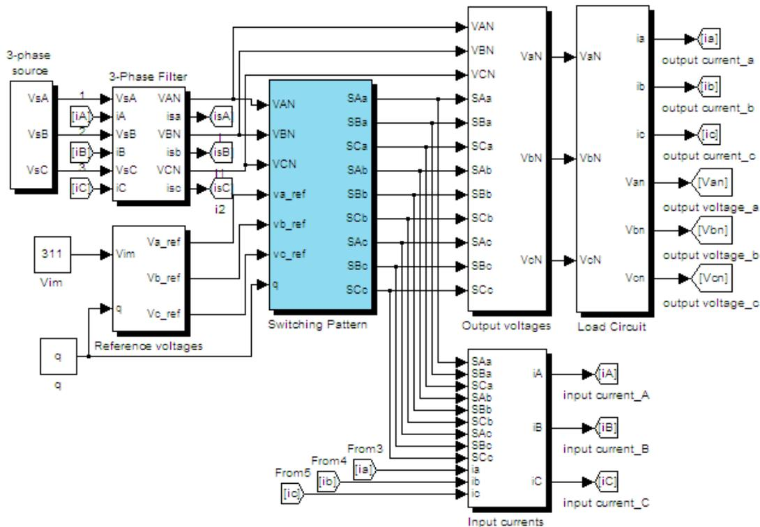
Fig.4. Matlab&Simulink model of the 3 x 3 matrix converter
