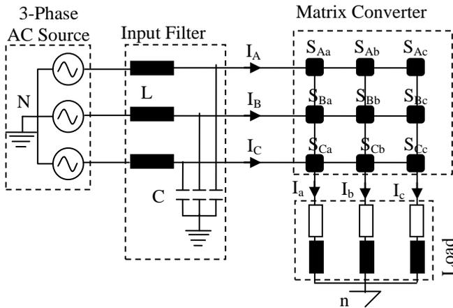
Fig. 1. Circuit of a 3 x 3 matrix converter
