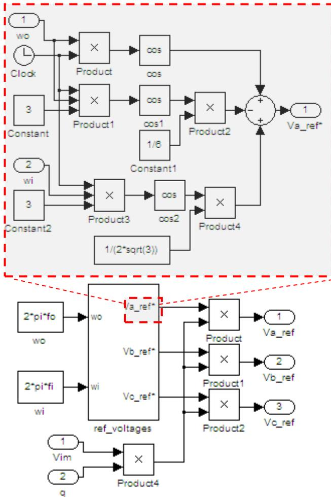
Fig. 2. Third-harmonic injection of the input and output frequencies into the output phase voltages
