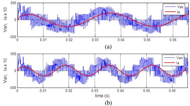
Fig. 7. Output phase voltage with respect to star point of load and output current: (a) in 30 Hz (b) in 60 Hz
