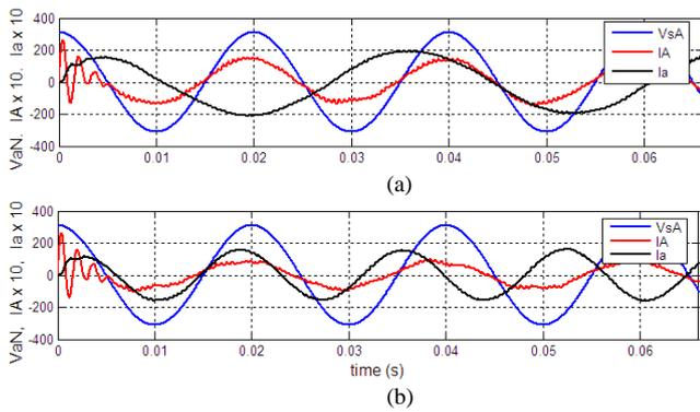
Fig. 9. Input voltage, input current and output current: (a) in 30 Hz (b) in 60 Hz
