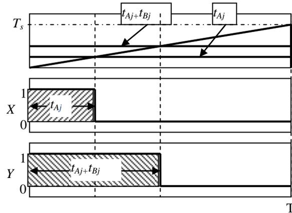
Fig.3. Gate signals of the power switches connected to the same output phase
