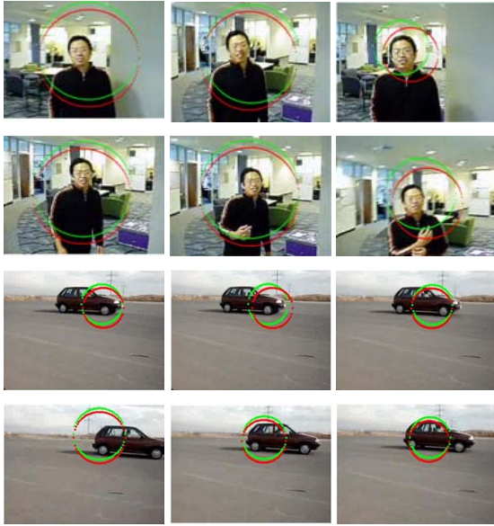
Fig. 3. Object tracking using the proposed method and the gravity center algorithm. The green circle is the tracked object based on the gravity center method and red circle is the tracked object based on the proposed method.
