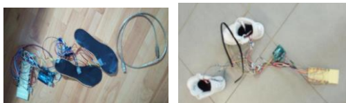
Fig. 13. Experimental setup for sensorial insoles with Arduino plate [18].
