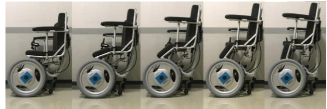
Fig. 7. Movement of the seat-lift mechanism.
