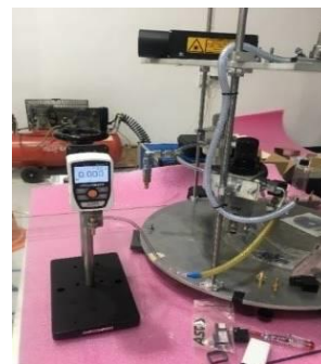
Fig. 5. Experimental setup for thruster static force measurement
