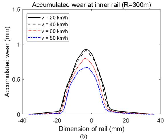
Fig. 4. Wear accumulation of the rails after about  $6 \times 10^5$  passages of the train under different train velocities: (a) left rail, (b) right rail.
