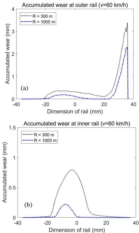
Fig. 6. Wear accumulation of the rails after about  $6 \times 10^5$  passages of the train under different track radii: (a) outer rail, (b) inner rail.
