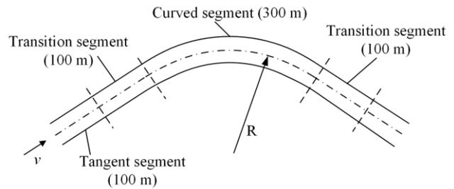
Fig. 2. The geometry of the curved track.
