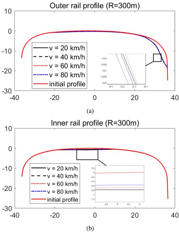
Fig. 3. Worn rail profiles after about  $6 \times 10^5$  passages of the train under different train velocities: (a) left rail, (b) right rail.
