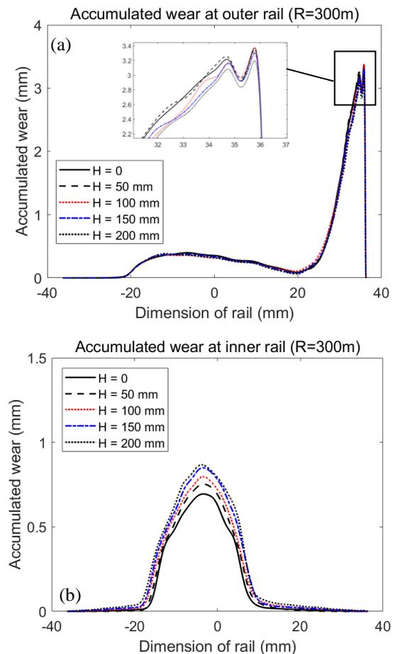
Fig. 7. Wear accumulation of the rails after about  $6 \times 10^5$  passages of the train under different track super-elevations: (a) outer rail, (b) inner rail.
