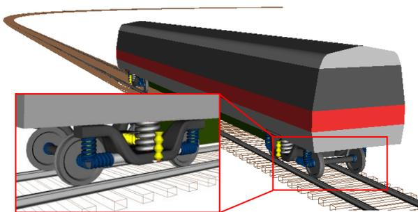
Fig. 1. Multibody vehicle/track model and suspension subsystem.
