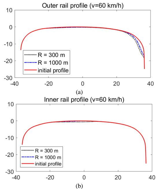
Fig. 5. Worn rail profiles after about  $6 \times 10^5$  passages of the train under different track radii: (a) outer rail, (b) inner rail.
