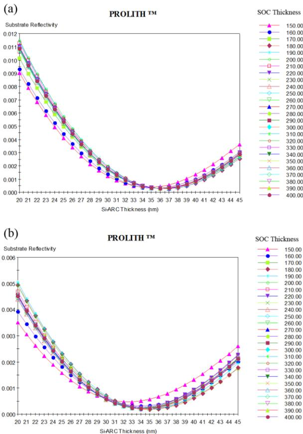
Fig. 2. The dependency of substrate reflectivity for the tri-layer stack on the thickness of SOC and Si-ARC. Using (a) cross-pole and (b) Quadropole illumination.
