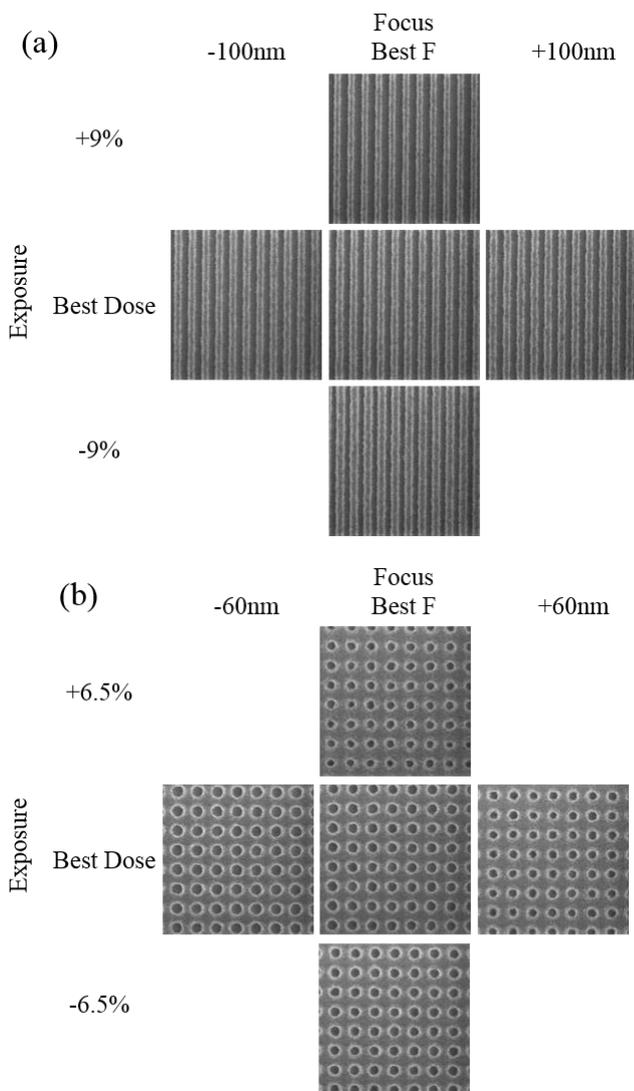
Fig. 6. The experimental focus exposure matrix (FEM) results of 45nm L/S and 65nm CH/130nm dense patterns developed by a tri-layer immersion process (1.3NA).
