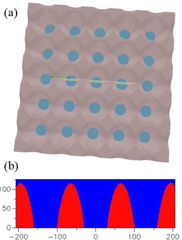
Fig. 5 (a) and (b) are the simulated 3D and cross-sectional resist profiles for the 65nm CH/130nm pitch dense patterns with a +30 nm CD mask bias.
