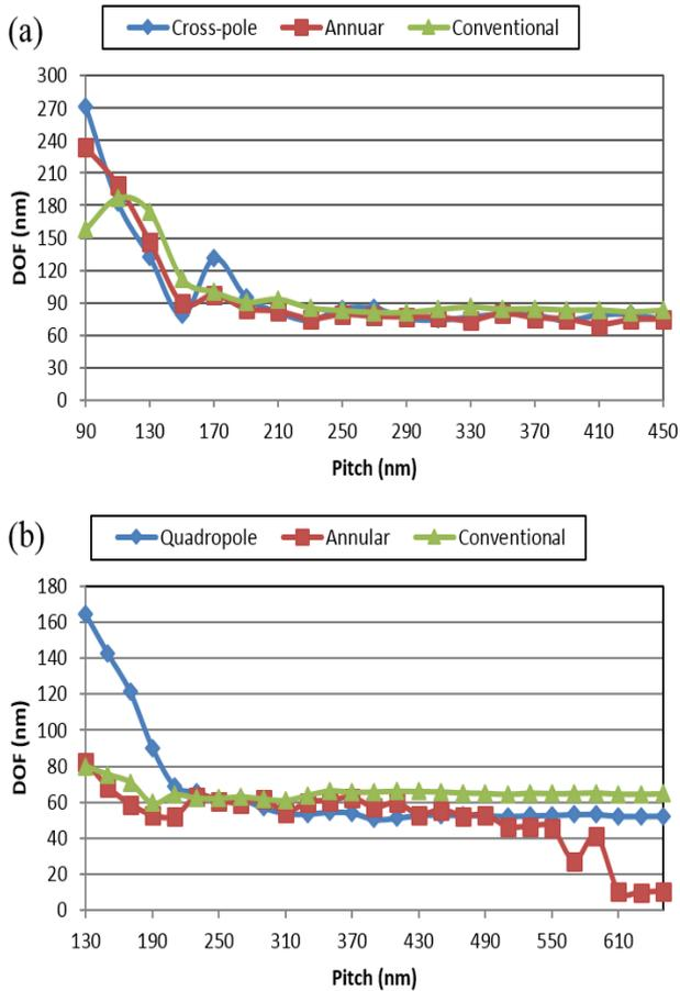
Fig. 4. The DOF performance of different illumination conditions to expose (a) 45nm line and (b) 65nm CH.
