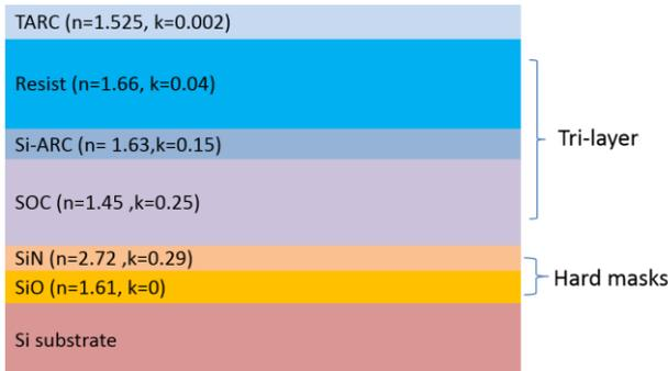
Fig. 1. A typical tri-layer stack on a silicon substrate with SiO and SiN hard masks.
