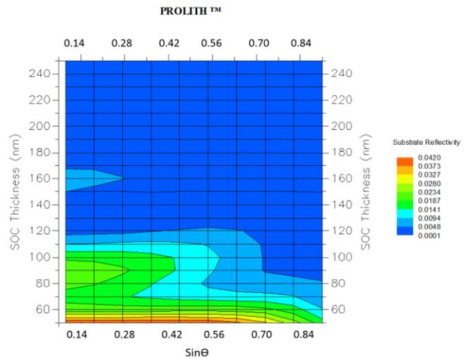
Fig. 3. The dependency of substrate reflectivity on the SOC thickness and the incident light angle.
