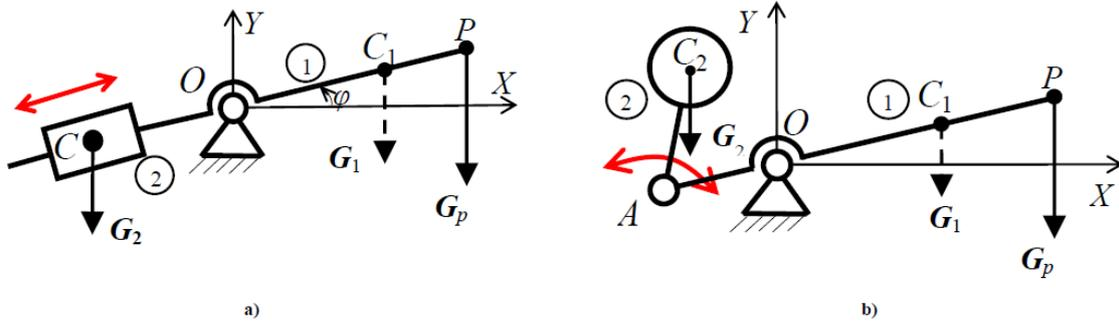
Fig. 3. Movable counterweight in order to compensate variable payload.
