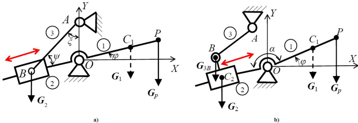
Fig. 4. Translatable counterweight in passive solution.
