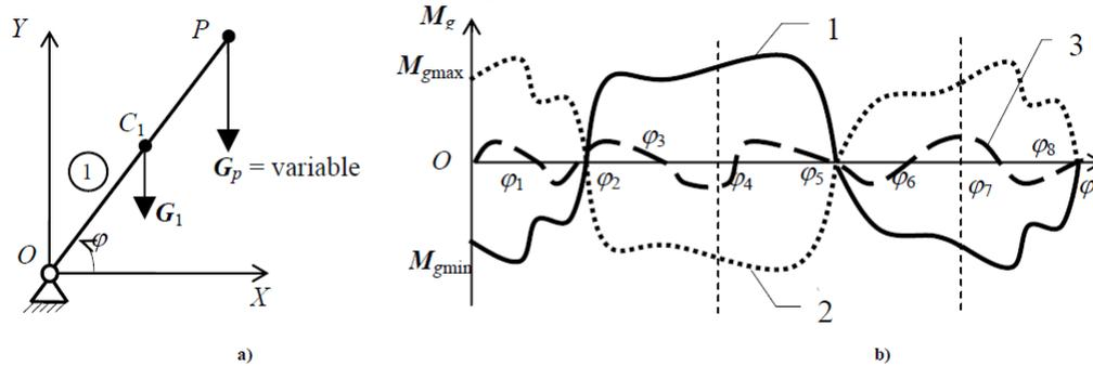
Fig. 1. Gravitational moment variation of the weight forces acted on an articulated arm.
