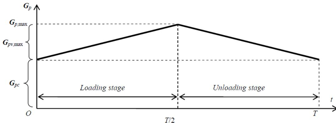
Fig. 2. Theoretic variation of a cyclic payload.
