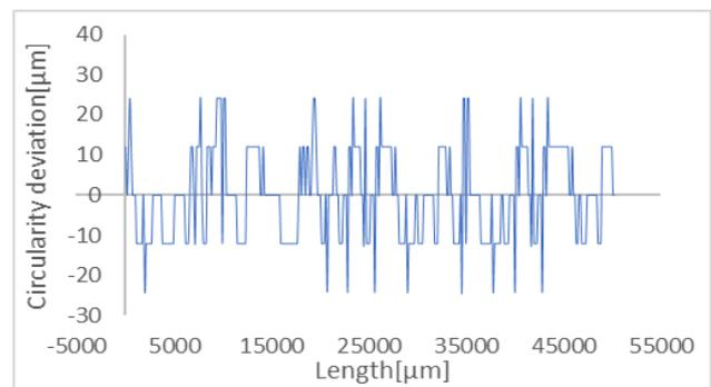
Fig. 12. Circularity deviation for inner ring.
