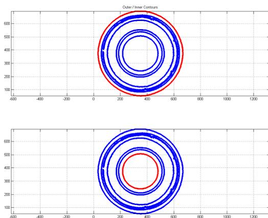
Fig. 10. Inner and outer ring contour definition.
