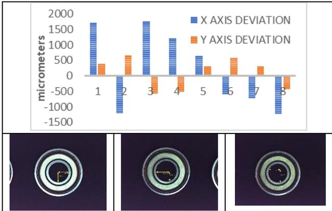
Fig. 5. Deviation from the center of the image.
