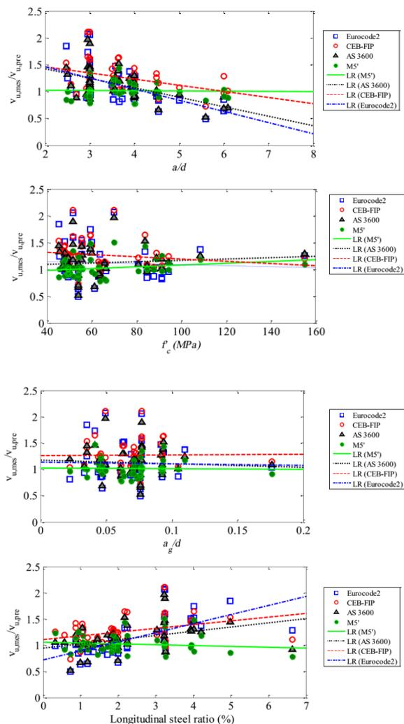
Fig. 4. Variation of discrepancy ratio (DR) between measured and predicted shear strength as a function of  $a/d$ ,  $a_g/d$ ,  $f_c$ , and  $\rho$ .
