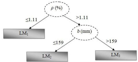
Fig. 1 Classification of dataset based on M5' algorithm.
