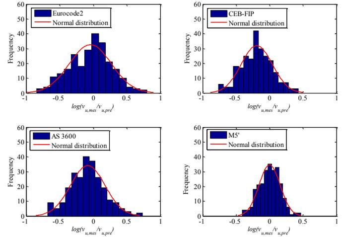
Fig. 3. Histograms of  $\log(v_{u,mes}/v_{u,pre})$  values for different approaches and their fitted normal distribution functions.
