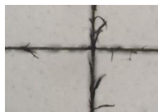
Fig. 2. FOW film burr on dicing tape.
