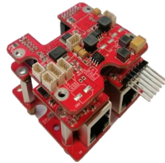
Fig. 14. Our developed high-voltage dynamic driver*.
