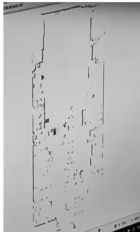
Fig. 17. Sample workspace map recorded by a LiDAR module, approx. 40m 2
