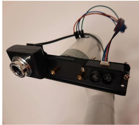
Fig. 13. Camera(left) and mini-testing LiDAR(right) attached to end effector of myCobot-Pi
