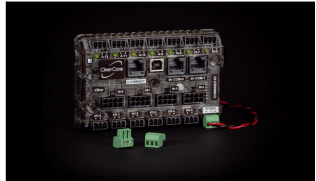
Fig. 3. ClearCore - Industrial motion and I/O controller [3]
