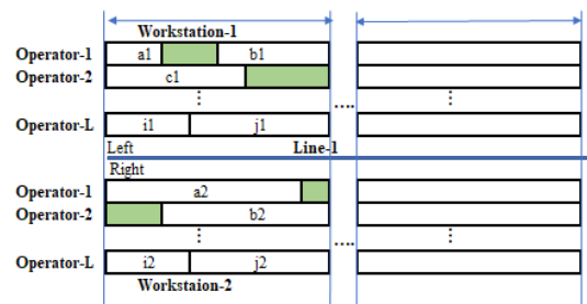
Fig. 1. Configuration of multi-manned two-sided assembly line.
