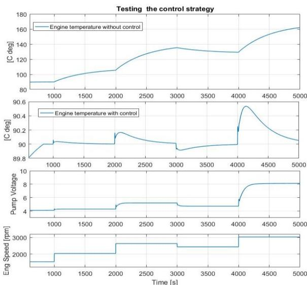
Fig. 7. Rejection of disturbances by the control system for different engine speeds.
