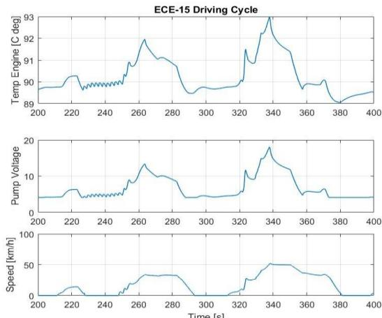
Fig. 8. Rejection of disturbances by the control system using ECE-15 driving cycle.
