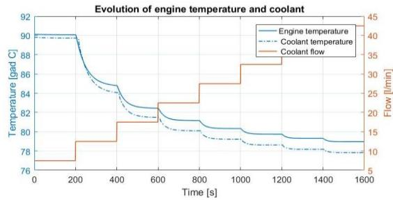
Fig. 4. Nonlinear behavior of motor temperature at different flow values.
