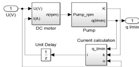
Fig. 3. The structure of the Simulink blocks used to model the pump.
