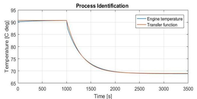
Fig. 6. Identify the transfer function used to calculate the controller.
