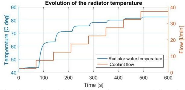
Fig. 5. The nonlinear behavior of the coolant temperature in the radiator at different flow values.
