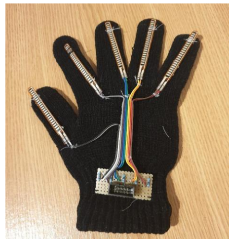
Fig. 4. Location of sensors on the glove.
