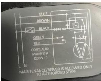
Fig. 4. Servomotor's wiring (detail view from the servomotor).
