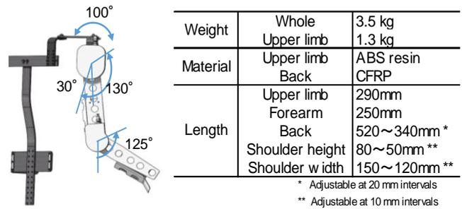
Fig. 3. Structure of the assist suit.
