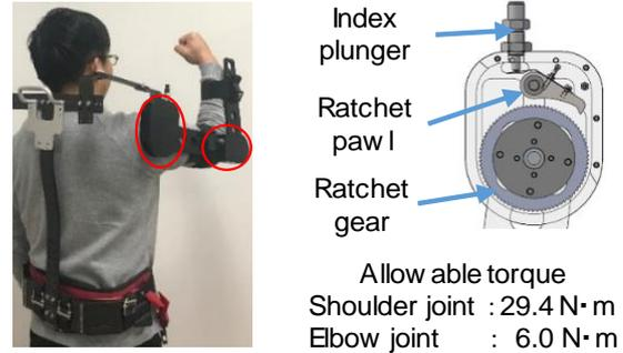
Fig. 4. Ratchet mechanism.
