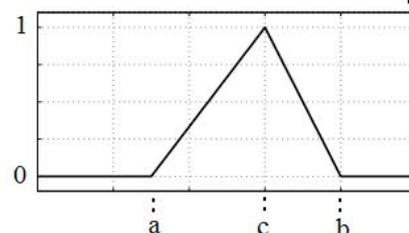
Fig. 2. A schematic representation of a triangular membership function
