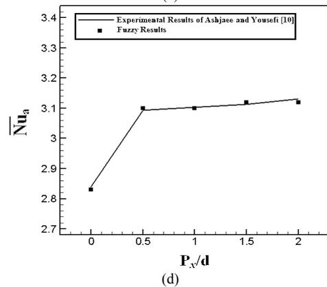
Fig. 13. Comparison between experimental and predicted values of average Nusselt number of the inclined array using ANFIS for a)  $Ra=10^3$  and  $P_y/d=2$  b)  $Ra=1.5 \times 10^3$  and  $P_y/d=3$  c)  $Ra=2.5 \times 10^3$  and  $P_y/d=4$  d)  $Ra=10^3$  and  $P_y/d=5$
