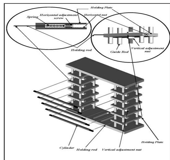
Fig. 5. Schematic of the holding stand of the cylinders and mechanisms for horizontal and vertical movement [10]
