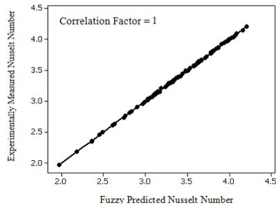
Fig. 11. The comparison between experimental and predicted values of average Nusselt number using fuzzy logic
