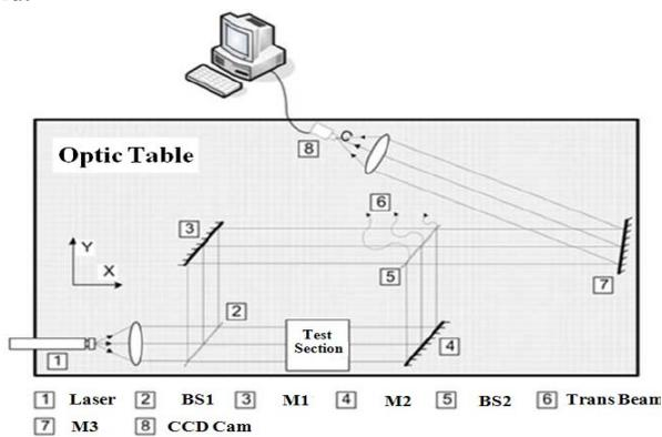
Fig. 3. Schematic of (MZI) setup [10]
