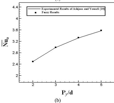
Fig. 12. Comparison between experimental and predicted values of average Nusselt number of the vertical array using ANFIS for a)  $Ra=1.5 \times 10^3$  b)  $Ra=2.5 \times 10^3$
