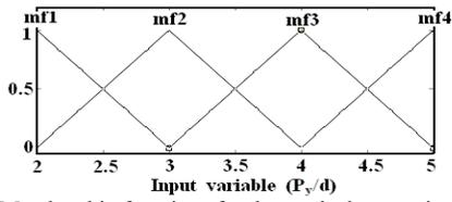
Fig. 8. Membership functions for the vertical separation distance
