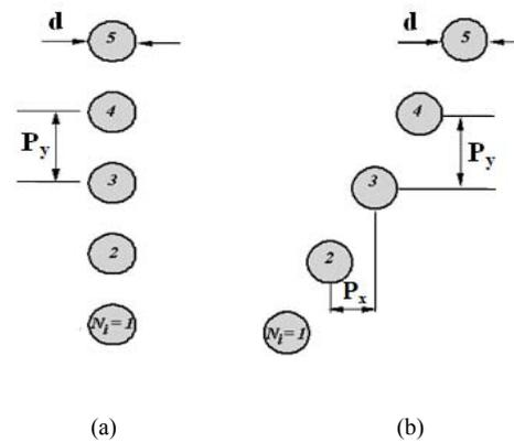
Fig. 1. Schematic representation of (a) the vertical array (b) the inclined array [10]
