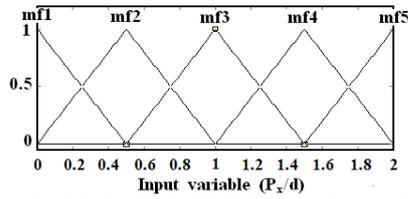
Fig. 9. Membership functions for the horizontal separation distance
