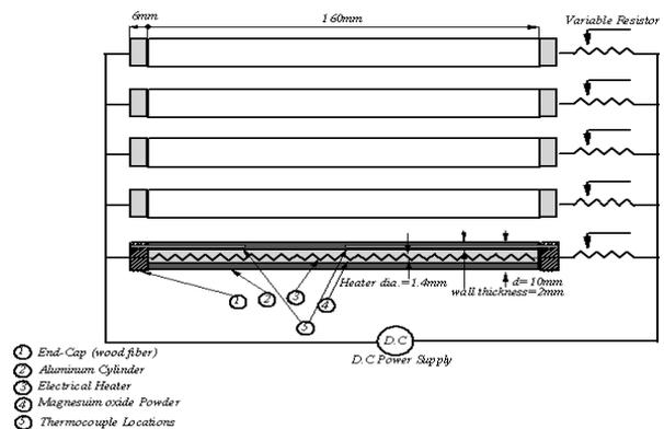
Fig. 4. Details of the cylinder used in the array with the heating circuit [10]
