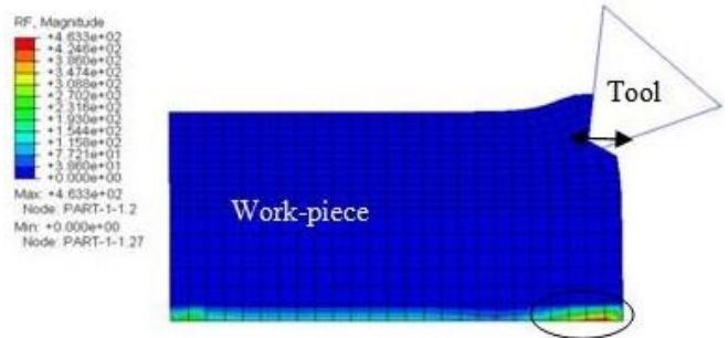
Fig. 2. Reaction force magnitude measured in the first frame at 80 m/min.
