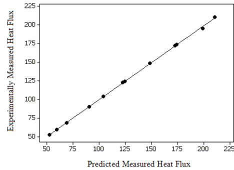
Fig. 8. The comparison between experimental and predicted values of average heat flux using ANFIS for training data.
