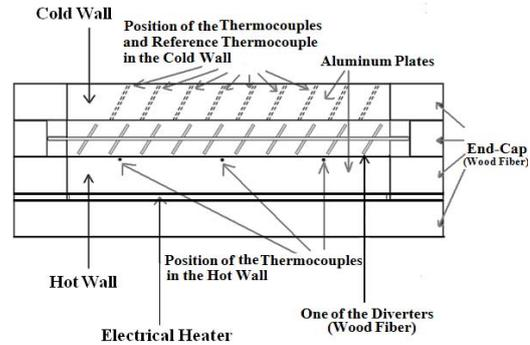
Fig. 4. Details of the horizontal cavity consisting of diverters used in the experiments.
