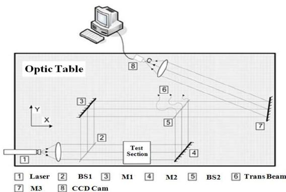
Fig. 2. Schematic representation of (MZI) setup.
