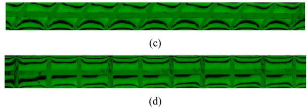
Fig. 3. Interferograms of the cavity consisting of diverters for  $Ra=12000$  at (a)  $\theta=0^\circ$  (b)  $\theta=30^\circ$  (c)  $\theta=60^\circ$  (d)  $\theta=90^\circ$ .
