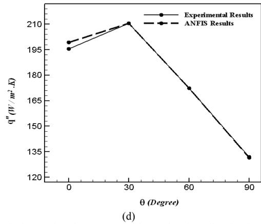
Fig. 10. Comparison between experimental and predicted values of convective heat flux using ANFIS for a) Ra=6000 b) Ra=8000 c) Ra=10000 d) Ra=12000.
