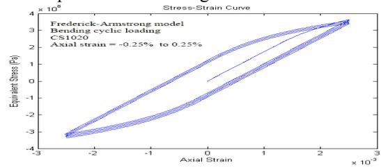
Fig. 8. Cyclic loading behavior for axial strain with zero mean, for a Frederick-Armstrong model.
