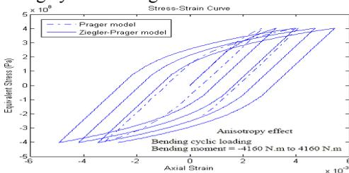
Fig. 7. Behavior of Euler-Bernoulli beam under cyclic flexural loading based on Prager and Ziegler-Prager models with material anisotropy.
