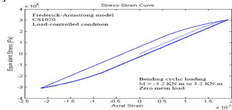
Fig. 9. Behavior of classical beam under symmetric cyclic loading.
