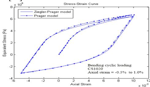
Fig. 5. Cyclic loading results on the beam with non-zero mean axial strain; comparison of Prager's, and its modified model.
