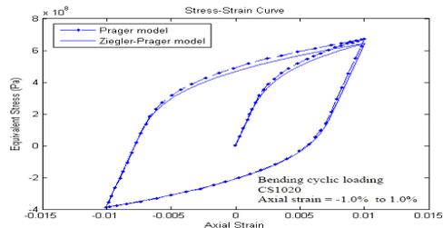
Fig. 4. Cyclic flexural loading with finite axial strain on *Euler-Bernoulli* beam; comparison of two models.
