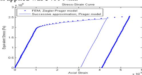
Fig. 1. Results of successive approximation method based on *Prager's* model and proposed FEM using *Ziegler-Prager* model.
