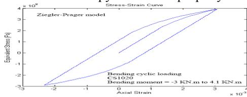
Fig. 6. Flexural loading on beam with non-zero mean stress.
