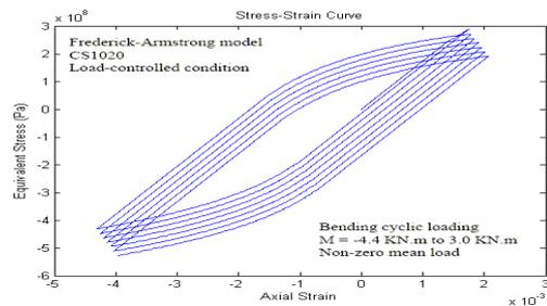
Fig. 10. Cyclic strain increase under asymmetric flexural loading based on Armstrong-Frederick yield surface movement model.
