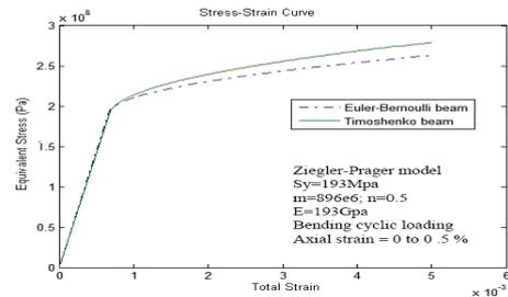
Fig. 3. Comparison of the behavior of Timoshenko beam with Euler-Bernoulli for strain controlled loading
