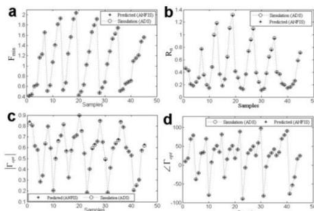
Fig. 2. The comparison between the simulation values and the predicted values using ANFIS model for testing data of : (a) Minimum noise figure, (b) Normalized equivalent resistance, (c) Magnitude of optimum reflection coefficient, (d) Angle of optimum reflection coefficient.
