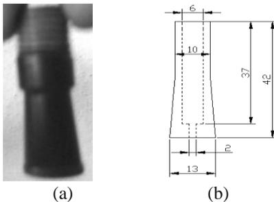
Figure 2: (a) Copper electrode with epoxy coating (b) Dimensions of the tool
