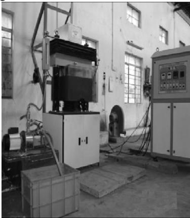
Figure 1: Electrochemical Machining setup
