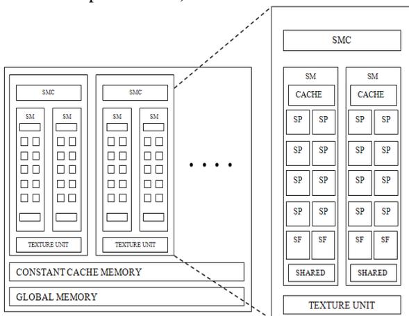
Fig. 1. Basic GPU architecture
