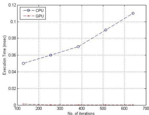
Fig. 3. GPU versus CPU Execution Time
