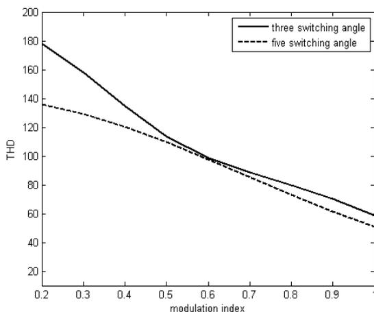
Fig. 8. THD versus modulation index for three and five switching angles
