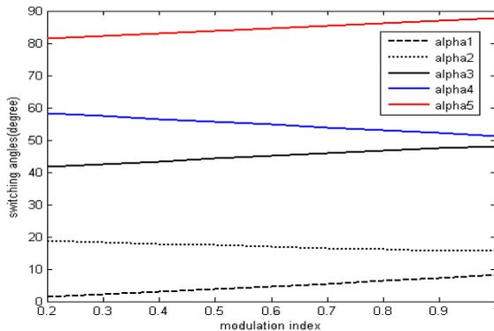
Fig. 7. Angle versus modulation index for five switching angles
