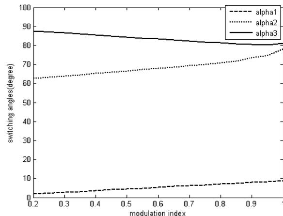
Fig. 4. Bipolar switching angles versus modulation index for three switching angles in PSO technique
