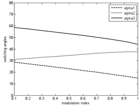
Fig. 3. Bipolar switching angles versus modulation index for three switching angles in Newton Raphson technique
