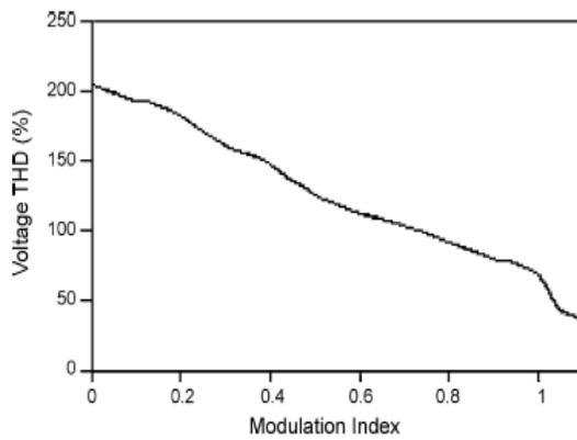
Fig. 5b. THD versus modulation index result of the previously reported PSO technique.
