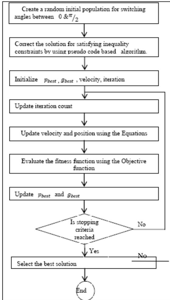
Fig. 2. Flowchart of PSO algorithm
