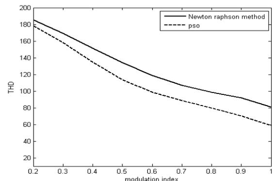
Fig. 5a. Comparison of THD between Newton Raphson and PSO method.
