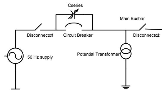
Fig. 1. System one line diagram arrangement resulting to PT ferroresonance [6]
