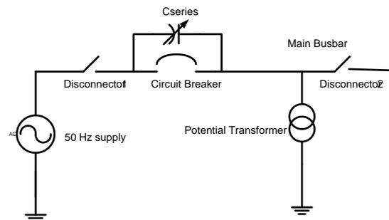
Fig. 1. System one line diagram arrangement resulting to PT ferroresonance [6]
