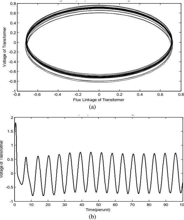
Fig. 5. (a) Phase plan diagram for quasiperiodic motion with neutral earth resistance effect and (b) Time domain simulation for quasiperiodic motion with neutral earth resistance effect
