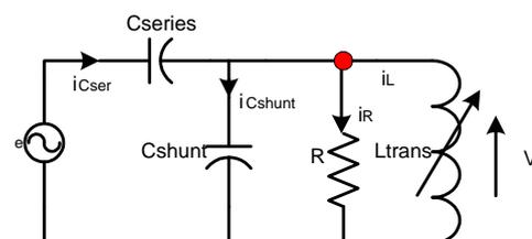
Fig. 2. Basic reduced equivalent ferroresonance circuit [6]
