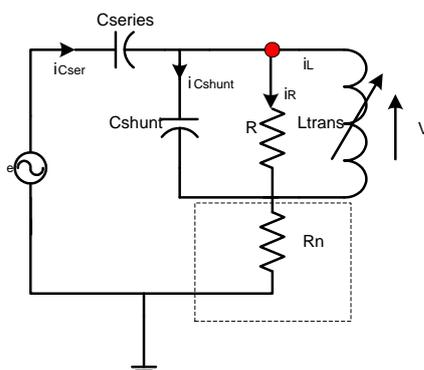
Fig. 3. Basic reduced equivalent ferroresonance circuit connecting neutral earth resistance
