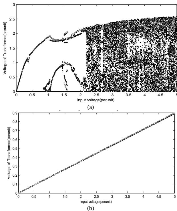
Fig. 6. (a) Bifurcation diagram for voltage of transformer versus voltage of system, without considering neutral earth resistance and (b) Bifurcation diagram for voltage of transformer versus voltage of system, with considering neutral earth resistance
