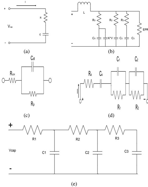
Fig. 1. (a) Simple UC Model (b) RC parallel branch model (c)UC Model with ESR and Rp (d) RC Branch Series – Parallel Model (e)Transmission line model
