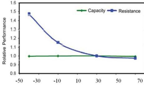
Fig. 2. Relative UC performance over operating temperature range From equation (4) and (5) after integration it can be written that:
