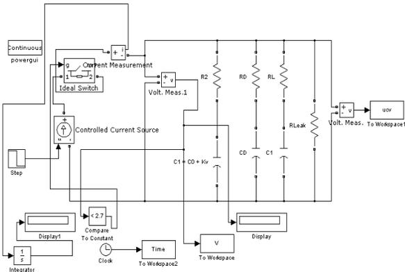
Fig. 4. MATLAB/Simulink model for both UC
