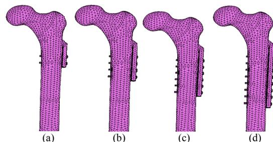
Fig. 1. The 3D FE models of the intertrochanteric fracture stabilized by various DHS; (a) 2-hole DHS, (b) 4-hole DHS, (c) 6-hole DHS, (d) 8-hole DHS
