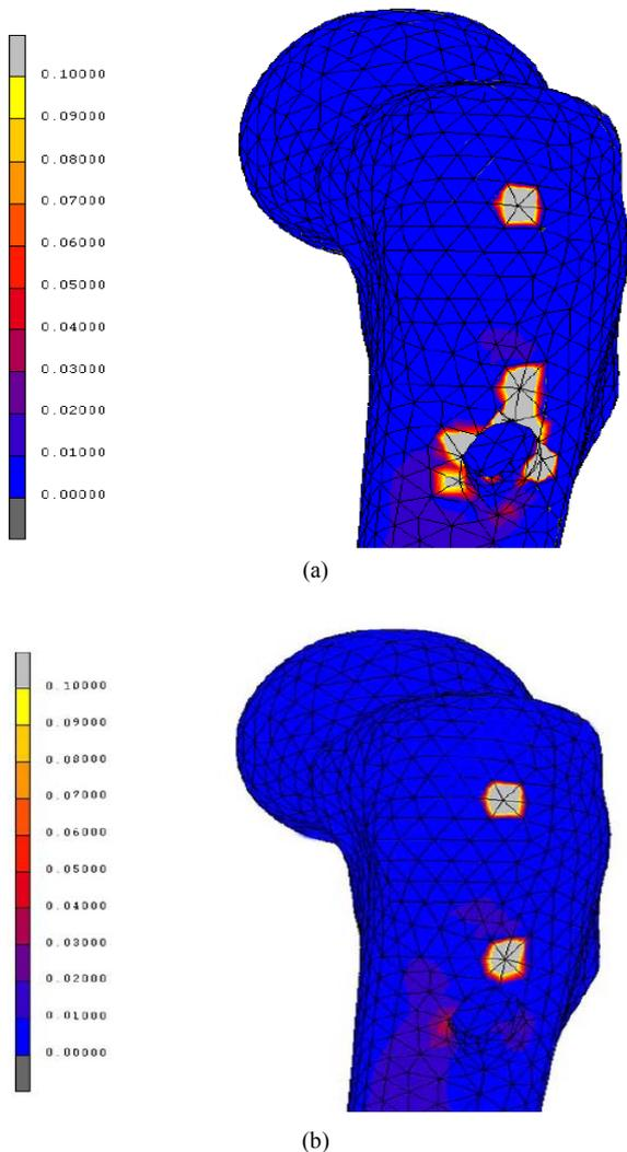
Fig. 6. The maximum SED at proximal shaft region inside DHS plate hole with: (a) retain of 2-hole DHS and (b) removal of 2-hole DHS
