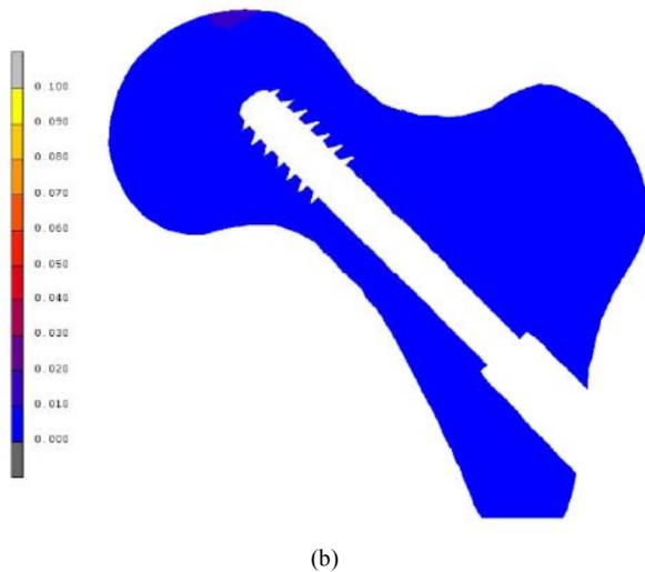
Fig. 5. The maximum SED at proximal neck cancellous region inside lag screw hole with: (a) retain of 2-hole DHS and (b) removal of 2-hole DHS
