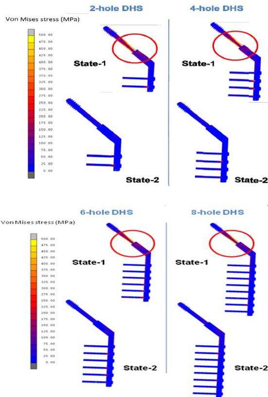
Fig. 4. The maximum von MISES stress on 2-hole DHS, 4-hole DHS, 6-hole DHS and 8-hole DH
