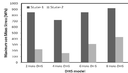
Fig. 3. The maximum von mises stress on the implants
